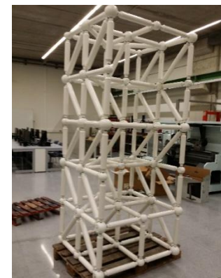
Prototype of the nodes/bars structure with integration of the hexapod (the actuators of the hexapod are not set)
